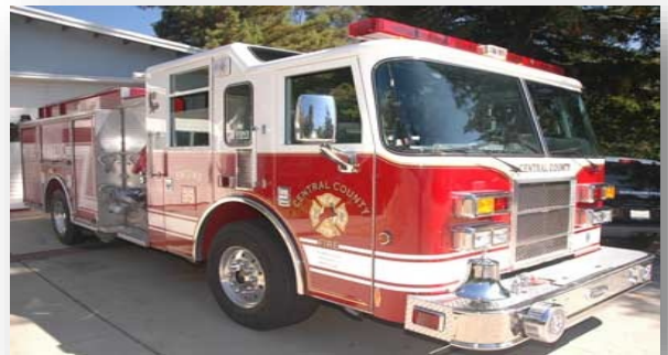
Engine 35 Pierce Dash Model Year 2000 Carries 680 gallons of water and 10 gallons each of Class A and Class B Foam
