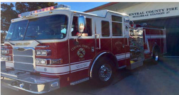
Engine 37 Pierce Dash Model Year 2016 Carries 680 gallons of water and 20 gallons of each Class A and Class B Foam
