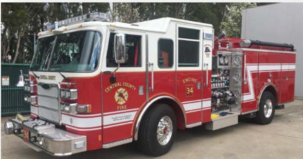
Engine 34 Pierce Dash Model Year 2016 Carries 680 gallons of water and 20 gallons of each Class A and Class B Foam
