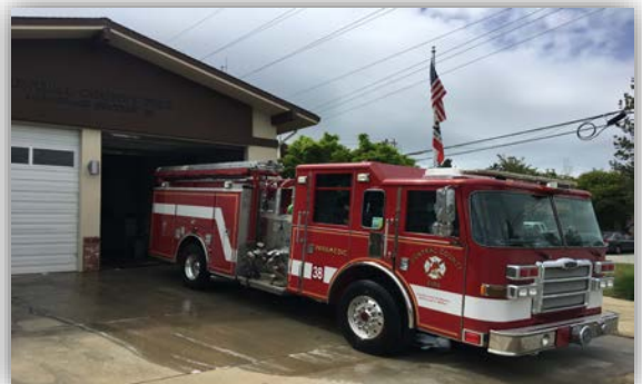
Engine 38 Pierce Dash Model Year 2002 Carries 680 gallons of water and 20 gallons of each Class A and Class B Foam
