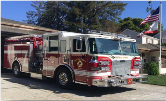
Engine 32 Pierce Dash Model Year 2016 Carries 680 Gallons of water and 20 gallons each of Class A and Class B Foam
