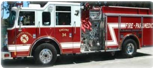
Engine 34 Pierce Dash Model Year 2002 Carries 680 gallons of water and 20 gallons of each Class A and Class B Foam
