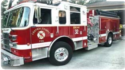
Engine 32 Pierce Dash Model Year 2002 Carries 500 Gallons of water and 20 gallons each of Class A and Class B Foam
