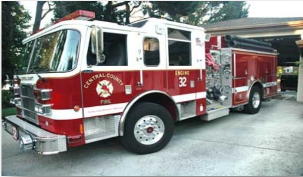
Engine 32 Pierce Dash Model Year 2002 Carries 500 Gallons of water and 20 gallons each of Class A and Class B Foam
