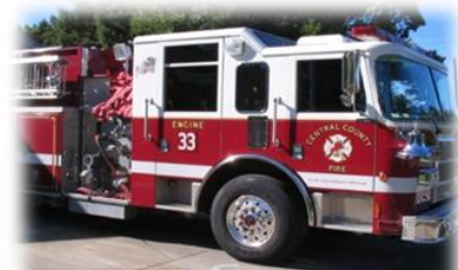
Engine 33 Pierce Dash Model Year 2002 Carries 500 gallons of water and 20 gallons of each Class A and Class B Foam
