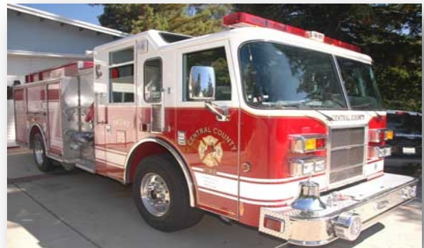
Engine 35 Pierce Dash Model Year 2000 Carries 680 gallons of water and 10 gallons each of Class A and Class B Foam
