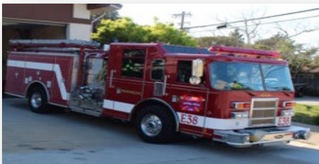
Engine 38 Pierce Dash Model Year 2002 Carries 680 gallons of water and 20 gallons of each Class A and Class B Foam
