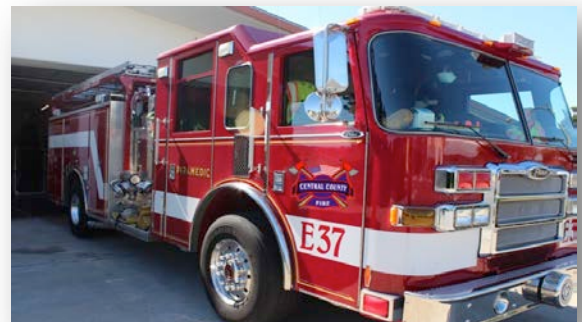
Engine 37 Pierce Dash Model Year 2002 Carries 680 gallons of water and 20 gallons of each Class A and Class B Foam
