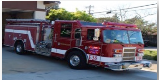
Engine 38 Pierce Dash Model Year 2002 Carries 680 gallons of water and 20 gallons of each Class A and Class B Foam
