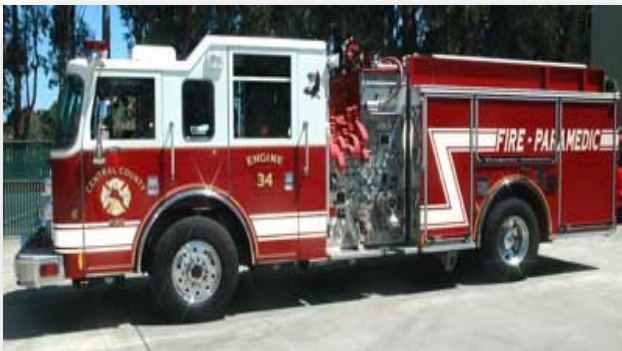
Engine 34 Pierce Dash Model Year 2002 Carries 680 gallons of water and 20 gallons of each Class A and Class B Foam
