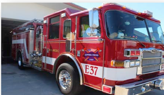
Engine 37 Pierce Dash Model Year 2002 Carries 680 gallons of water and 20 gallons of each Class A and Class B Foam
