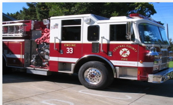
Engine 33 Pierce Dash Model Year 2002 Carries 500 gallons of water and 20 gallons of each Class A and Class B Foam
