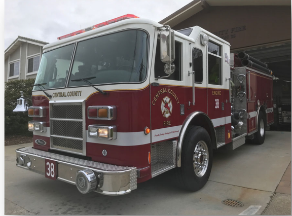
Engine 38 Pierce Dash model year 2002 Carries 680 gallons of water and 20 gallons each of Class A and Class B foam
