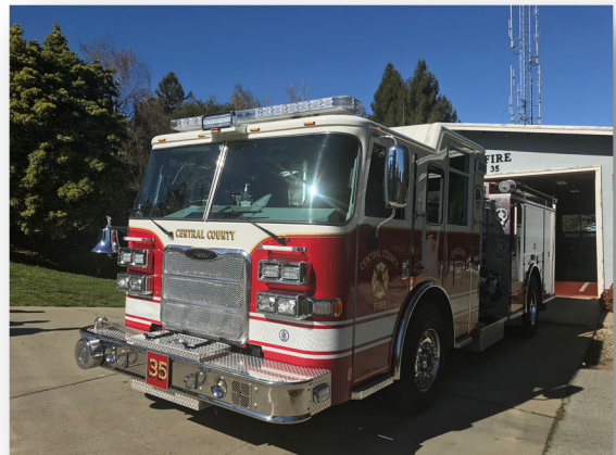
Engine 35 Pierce Dash model year 2000 Carries 680 gallons of water and 20 gallons of universal foam
