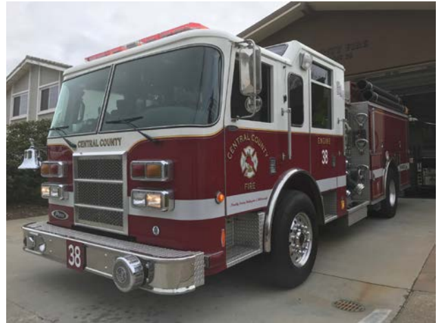
Engine 38 Pierce Dash model year 2017 Carries 680 gallons of water and 20 gallons each of Class A and Class B foam
