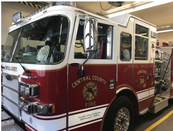
Engine 34 Pierce Dash model year 2016 Carries 680 gallons of water and 20 gallons of universal biodegradable foam
