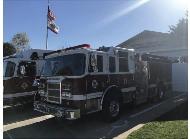
Engine 33 Pierce Dash model year 2002 Carries 500 gallons of water and 20 gallons each of Class A and Class B foam
