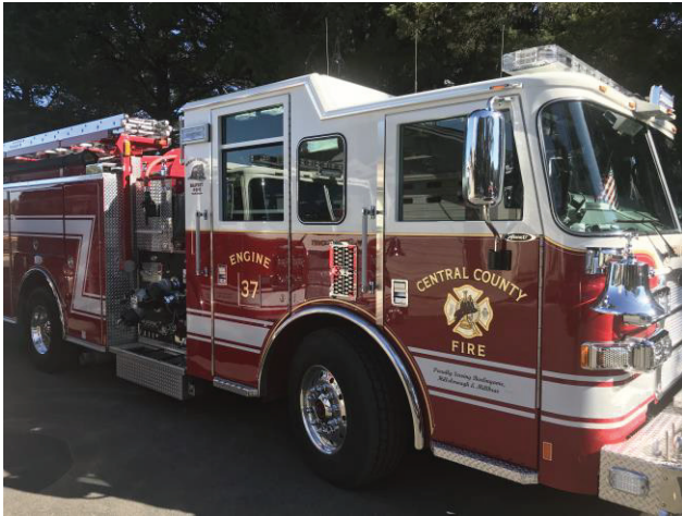
Engine 37 Pierce Dash model year 2017 Carries 680 gallons of water and 20 gallons of universal biodegradable foam
