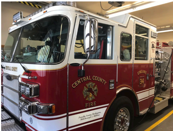
Engine 34 Pierce Dash model year 2019 Carries 680 gallons of water and 20 gallons of universal biodegradable foam
