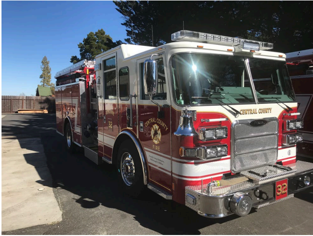
Engine 32 Pierce Dash model year 2016 Carries 680 gallons of water and 20 gallons of universal biodegradable foam
