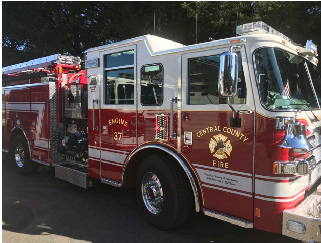
Engine 37 Pierce Dash model year 2016 Carries 680 gallons of water and 20 gallons of universal biodegradable foam
