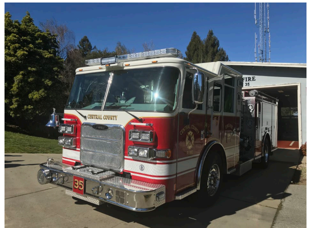
Engine 35 Pierce Dash model year 2016 Carries 680 gallons of water and 20 gallons of universal biodegradable foam
