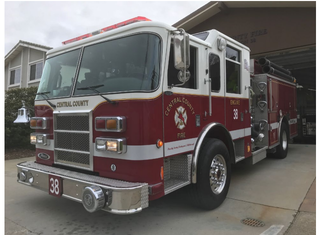
Engine 38 Pierce Dash model year 2017 Carries 680 gallons of water and 20 gallons of universal biodegradable foam
