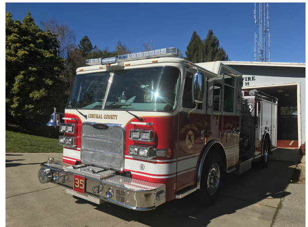
Engine 35 Pierce Dash model year 2002 Carries 500 gallons of water and 20 gallons of universal foam
