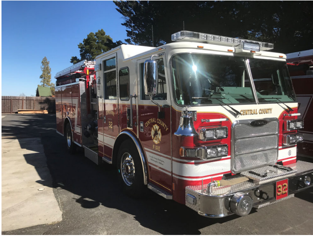
Engine 32 Pierce Dash model year 2017 Carries 680 gallons of water and 20 gallons of universal foam
