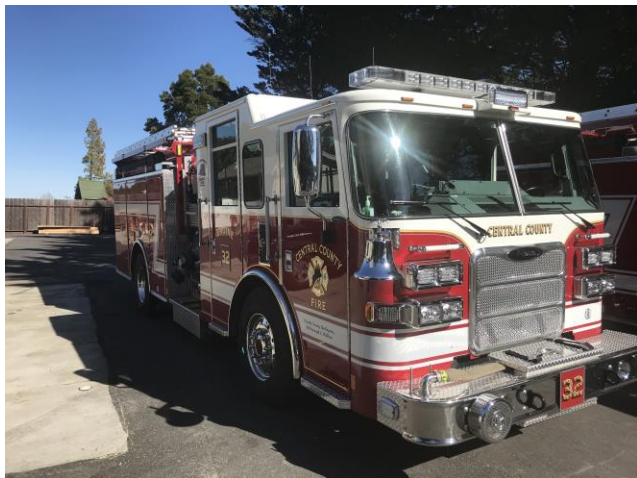
Engine 32 | Pierce Dash model year 2016 Carries 680 gallons of water and 20 gallons of universal foam
