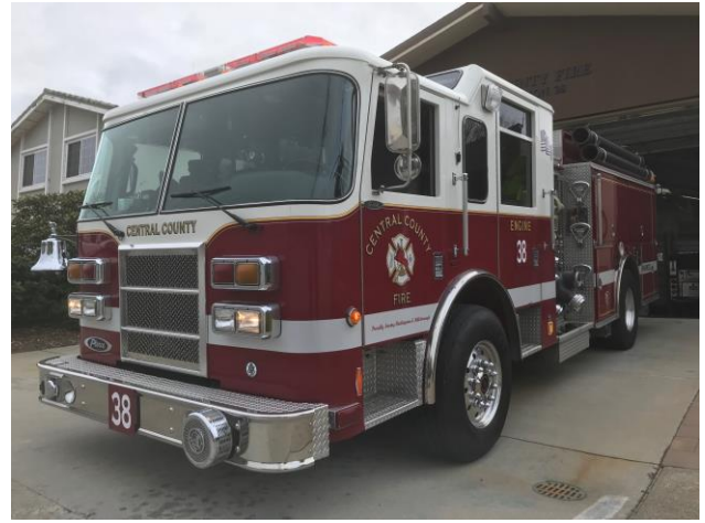
Engine 38 | Pierce Dash model year 2017 Carries 680 gallons of water and 20 gallons each of universal biodegradable foam
