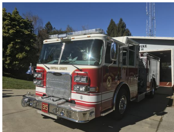
Engine 35 | Pierce Dash model year 2016 Carries 680 gallons of water and 20 gallons of universal biodegradable foam
