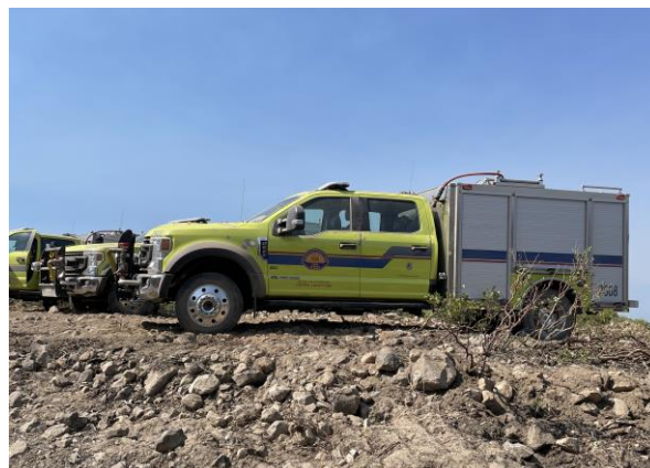
Engine 2608 | 2020 Ford HME/Ahrens-Fox CA Office of Emergency Services Type 6 Apparatus
